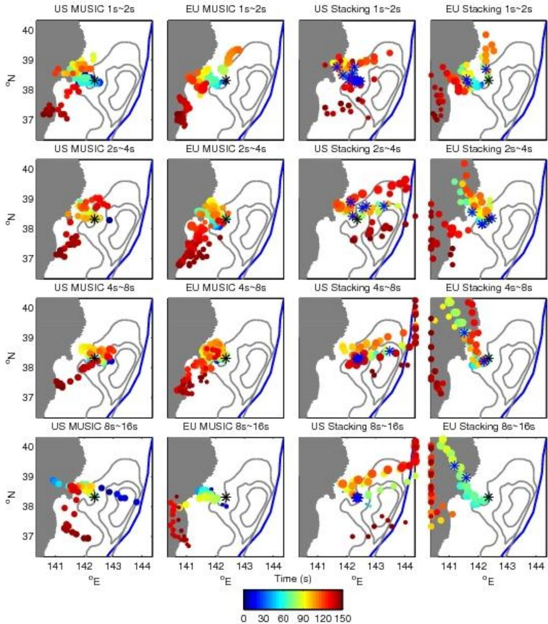
**Figure 6** back-projection of the Tohoku-Oki earthquake at various periods (1s~16s) of USArray and European array data with the linear stacking and MUSIC approaches. The
