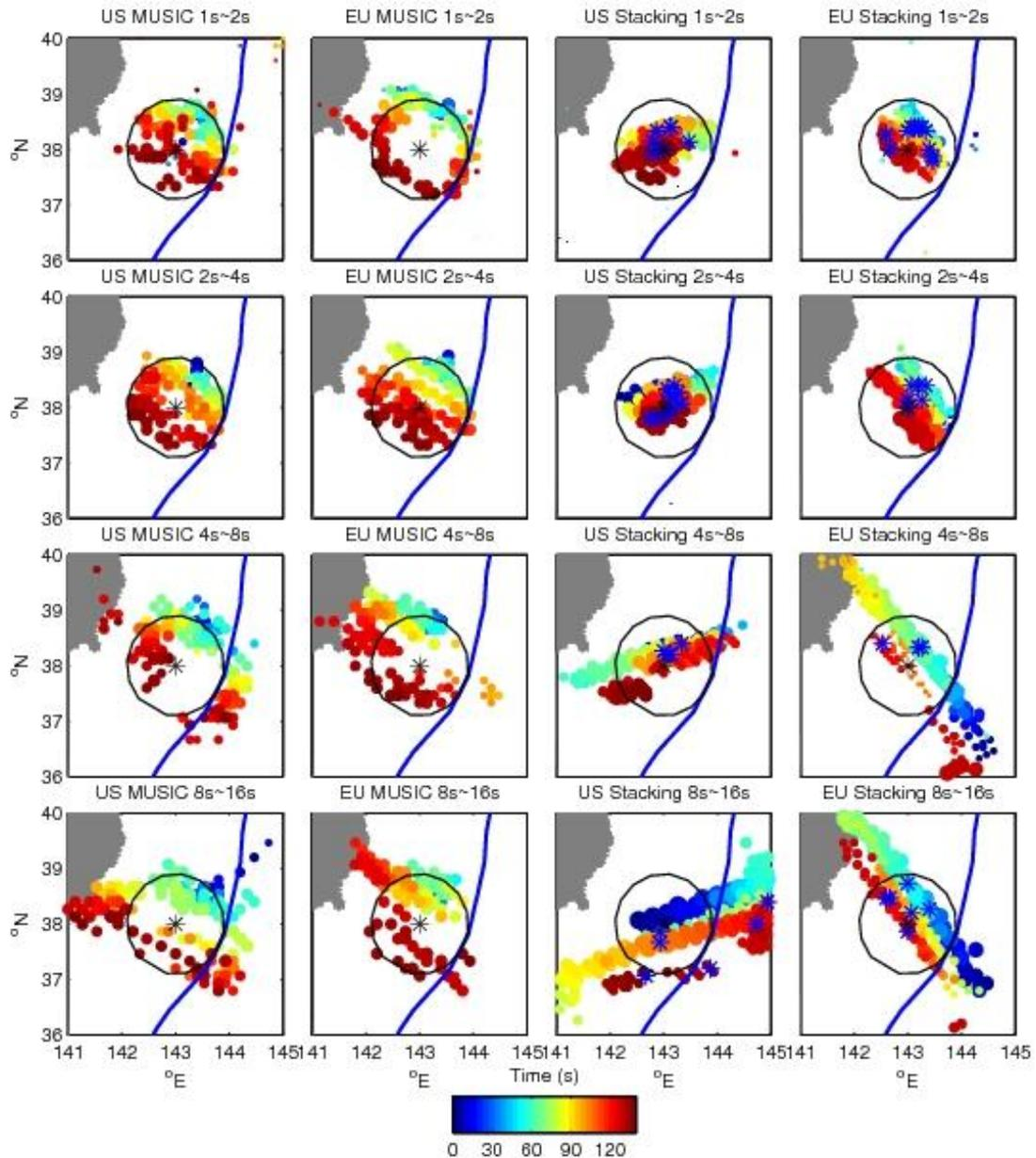
**Figure 5 Back-projection of circular rupture synthetics.** The synthetic seismograms of a circular rupture scenario recorded at USArray (left two columns) and European array (right two
