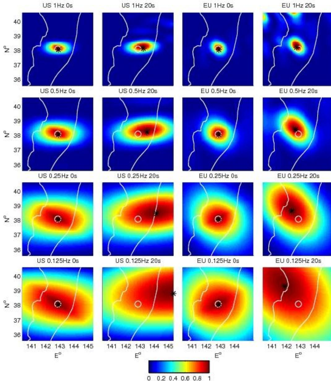
**Figure 2** Swimming effect in the 2D array response of the USArray (left two columns) and European array (right two columns) at frequency of 1, 0.5, 0.25 and 0.125 Hz, with color coded
