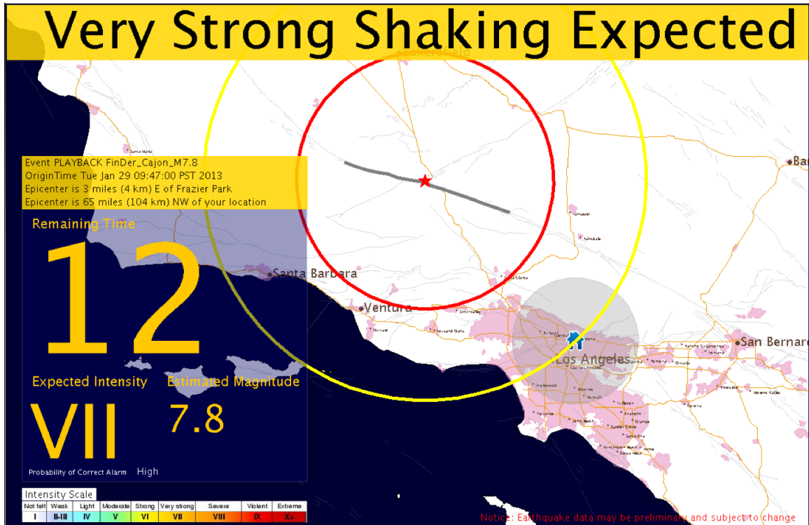
Finite fault detection capability of EEWDisplay. Thick grey line shows extent of current fault rupture.
