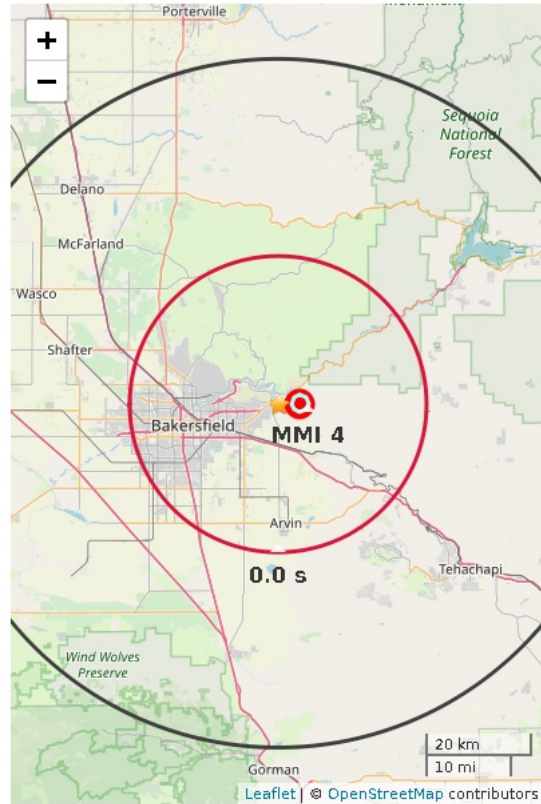
Figure 1. ShakeAlert earthquake location (red dot). Star is regional network epicenter. Polygon is the predicted outer range for felt ground motion (MMI 2). Red circle is locus of peak shaking when the alert was released. Shaking takes 10 s to expand from circle to circle.
