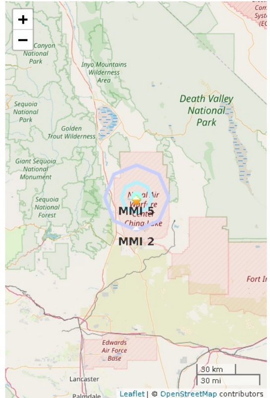
Figure 2. Polygons show shaking intensity contours for the final ShakeAlert. Shaking of intensity 3 or less is often not felt. Star shows the regional network epicenter.
