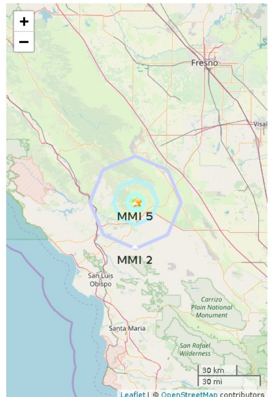
Figure 2. Polygons show shaking intensity contours for the final ShakeAlert. Shaking of intensity 3 or less is often not felt. Star shows the regional network epicenter.
