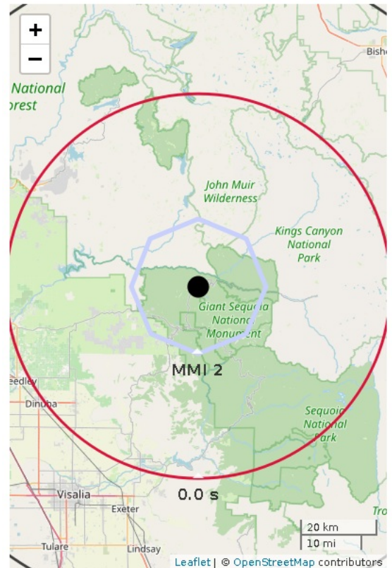
Figure 1. ShakeAlert initial earthquake location (black dot). Regional network epicenter not available. Polygon is the predicted outer range for felt ground motion (MMI 2). Red circle is front of peak shaking when the alert was released. Shaking takes 10 s to expand from circle to circle.
