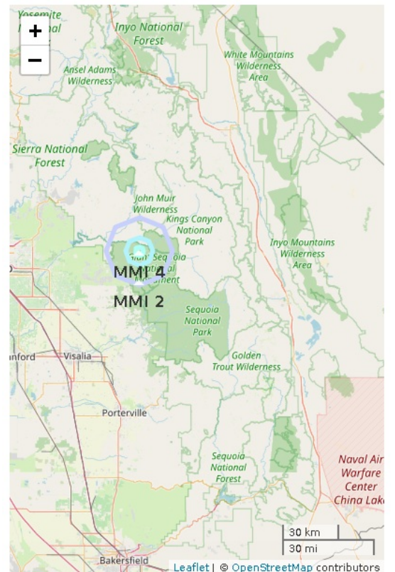
Figure 2. Polygons show shaking intensity contours for the peak magnitude ShakeAlert. Shaking of intensity 3 or less is often not felt. Regional network epicenter not available.
