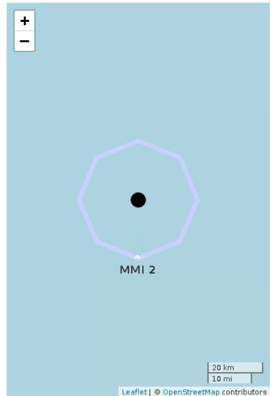
Figure 1. ShakeAlert initial earthquake location (black dot). Regional network epicenter not available. Polygon is the approximate outer range for felt ground motion. If shown***, red circle is front of peak shaking when the alert was released. Shaking takes 10 s to expand from circle to circle.
