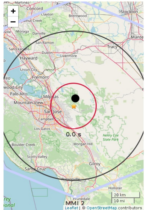
Figure 1. ShakeAlert initial earthquake location (black dot). Star is regional network epicenter. Polygon is the approximate outer range for felt ground motion. If shown***, red circle is front of peak shaking when the alert was released. Shaking takes 10 s to expand from circle to circle.
