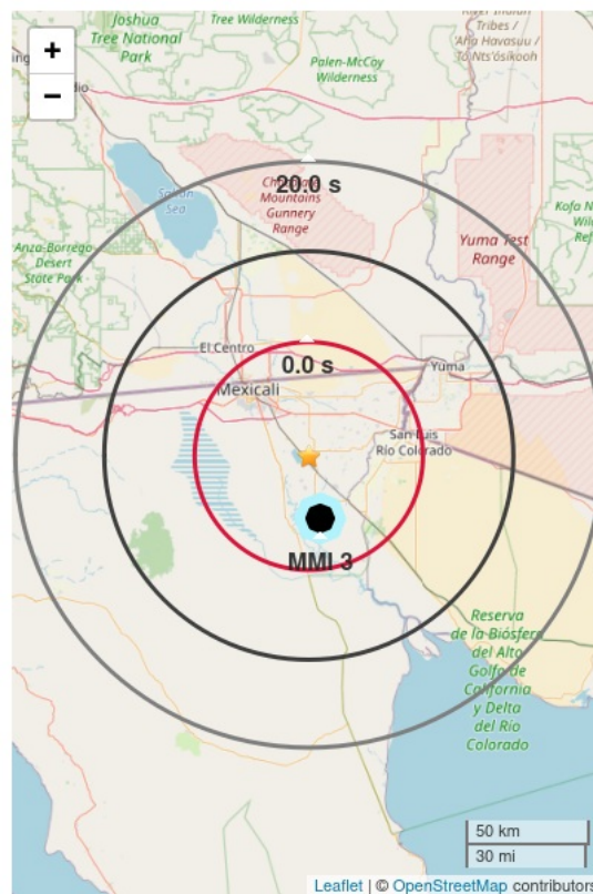
Figure 1. ShakeAlert initial earthquake location (black dot). Star is ANSS earthquake epicenter. Polygon approximates the outer range for felt ground motion. If shown, red circle is front of peak shaking when the Message was released***. Shaking takes 10 s to expand from circle to circle.
