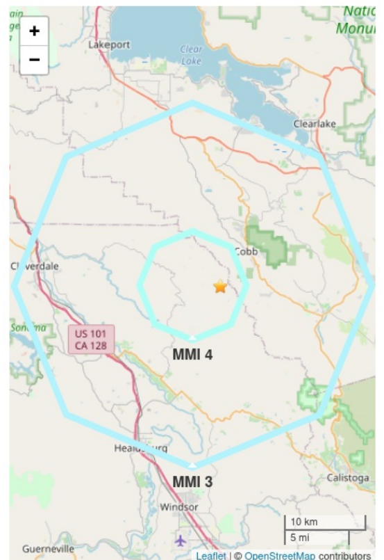
Figure 2. Polygons show the largest contours of estimated shaking intensity. Shaking of MMI 3 or less is often not felt. Star shows the ANSS earthquake epicenter.
