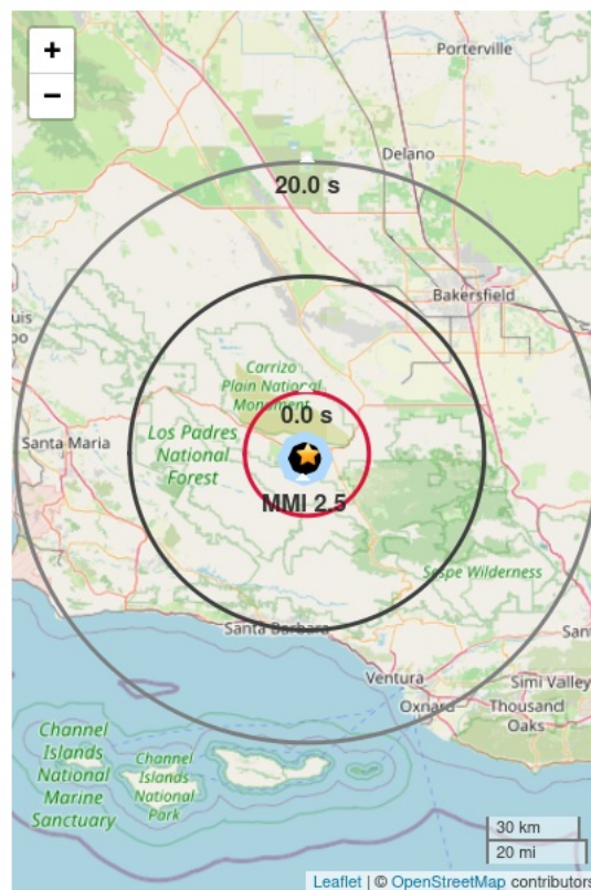
Figure 1. Initial earthquake locations from ShakeAlert (black dot) and ANSS (orange star). Polygon shows estimated area of felt ground shaking**. Red circle (if shown) marks the position of the peak shaking wave front at the time the Alert Message was issued***. Note, shaking takes 10 seconds to expand from circle to circle.
