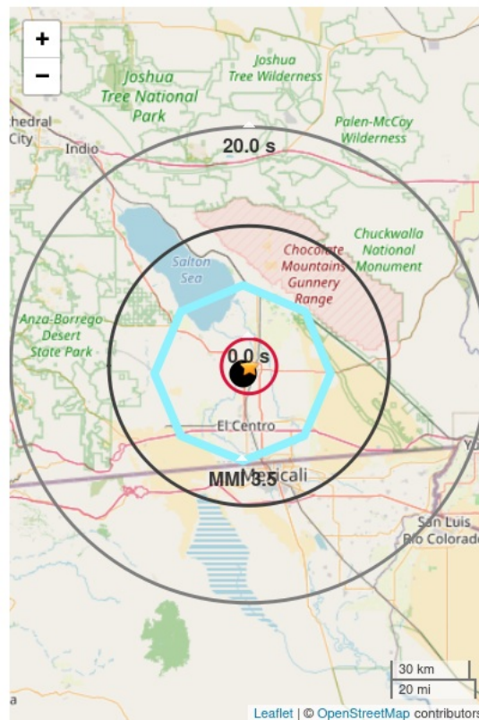
Figure 1. Initial earthquake locations from ShakeAlert (black dot) and ANSS (orange star). Polygon shows estimated area of MMI 3.5 and greater ground shaking**. Red circle (if shown) marks the position of the peak shaking wavefront at the time the Alert Message was issued***. Note, shaking takes 10 seconds to expand from circle to circle.
