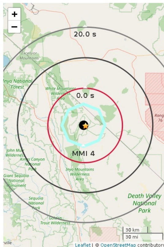
Figure 1. ShakeAlert initial earthquake location (black dot). Star is ANSS earthquake epicenter. Polygon shows estimated MMI 4 shaking intensity area. If shown, red circle is front of peak shaking when the message was released***. Shaking takes 10 s to expand from circle to circle.
